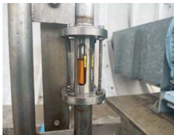
Pict. 21 Lube oil on max level in sight glass.
