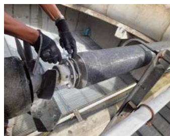
Pict. 12 Check coupling gap after final alignment.
