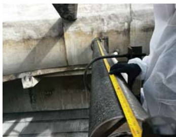
Pict. 13 Check distance between shaft ends after.
