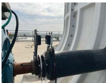
Pict. 8 Adjust drive shaft alignment after motor.
