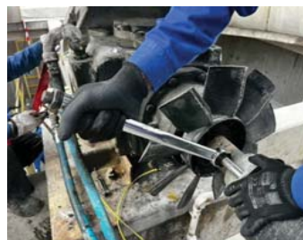
Pict. 11 Tighten torque bolt of drive shaft coupling gearbox.
