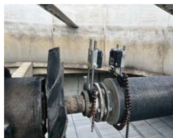
Pict. 9 Adjust drive shaft alignment after gearbox.
