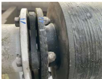
Pict. 22 Inspection flexible element of coupling.
