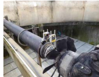
Pict. 9 Adjust drive shaft alignment after gearbox.
