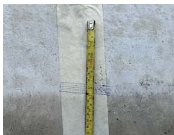
Pict. 16 Check fan blade tip track after tighten torque bolt.
